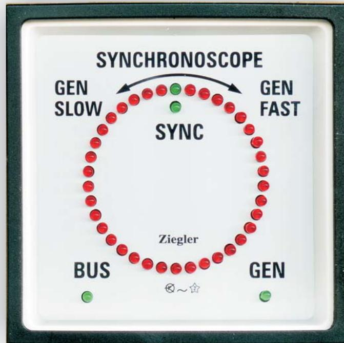
The Electronic Synchroscope is Designed to Provide an Illuminated Indication of Actual Phase Difference Between the BUS Voltage (Reference Voltage) and the GENERATOR Voltage (Incoming Voltage).
